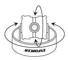
Remove the dome (see page 3, Installation) and adjust the pan or tilt of the Indoor Mini Dome Camera by hand.
